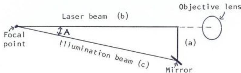
Example: Tangent of angle  $A = a$  divided by  $b$ ; or, for example,  $9.8 / 62$ , or  $0.1584$ . From the trigonometry tables, that equals a 9 degree angle.
