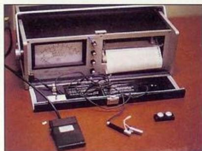
**Machine with electronic tonometer, standardization block and foot pedal for classic tonography.**
